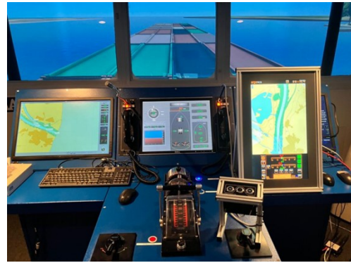
Figure 1: One of the bridge simulators used in the project. The interface of the trackpilot of Argonics is right on the picture.
