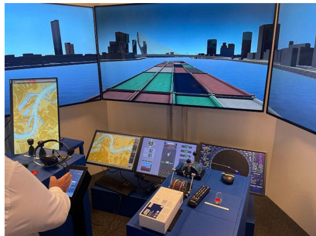
Figure 2: Bridge simulator at MARIN. The trackpilot of Shipping Technology as well as an alternative visualization are on the left.
