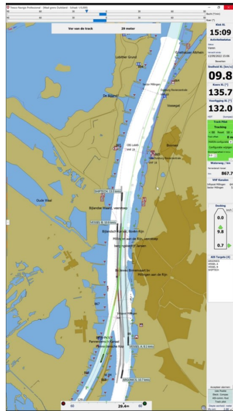
Figure 3: Intentions shown on an Inland ECDIS system of TRESCO Engineering.
