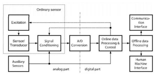
Figure 2: Intelligent sensor structure (Automationforum.co)
