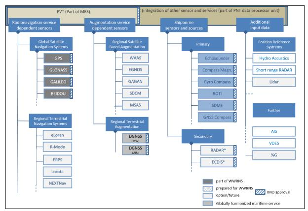
Figure 5: Sensors Services and sources to Provide PNT on board vessels 2
