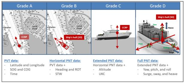
Figure 4: Application Grades of PNT-DP<sup>2</sup> (\*provided with improved accuracy)
