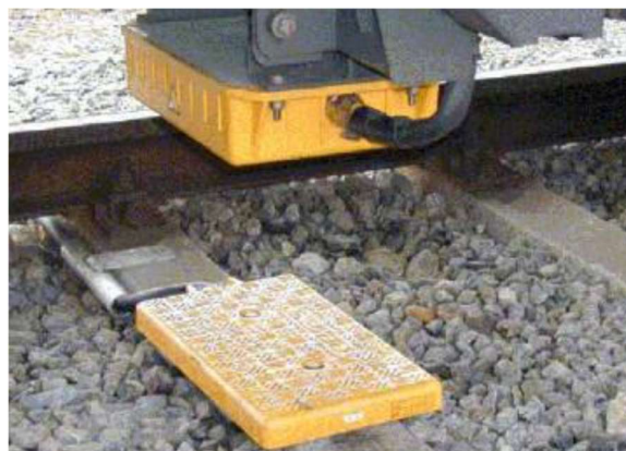
Figure 11: Example of railway balise
