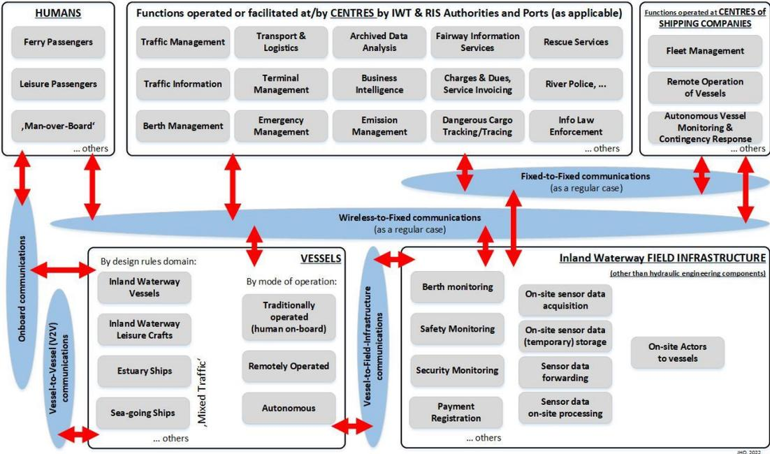
Figure 14: IWT Fairway & Navigation System Interconnection Architecture (ISIA)
